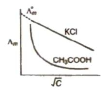
The limiting value,  $\Lambda^0_{m}$  or  $\Lambda^\infty_{m}$ . (the molar conductivity at zero concentration (or at infinite dilution) can be obtained extrapolating the graph.
